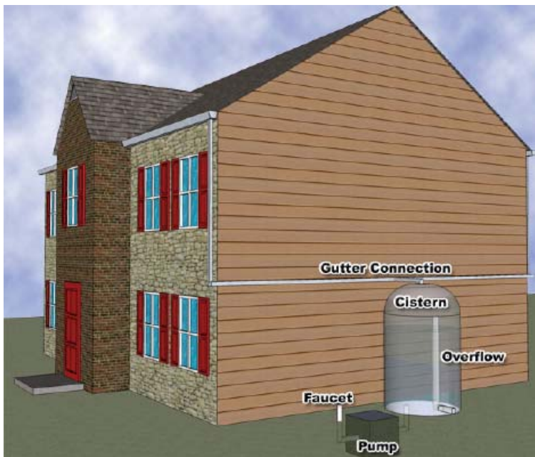
Figure 1 Basic rainwater harvesting system components.
