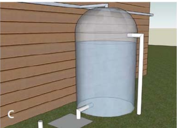
Figure 6 A, B, C. Basic overflow configuration
