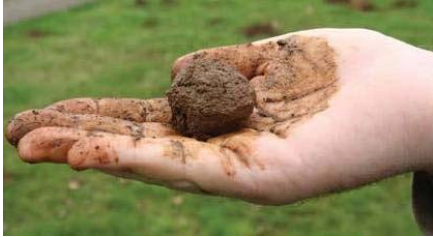
Figure 4 Soil texture assesses organic content and soil type. Step 3 is shown here.
