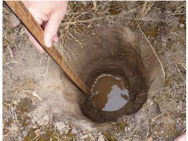
Figure 3 A shovel was used to dig most of the way then a 6" diameter post hole digger was used to reach the proposed bottom elevation of a rain garden. Measure the drop in water from a known, stable marker.
