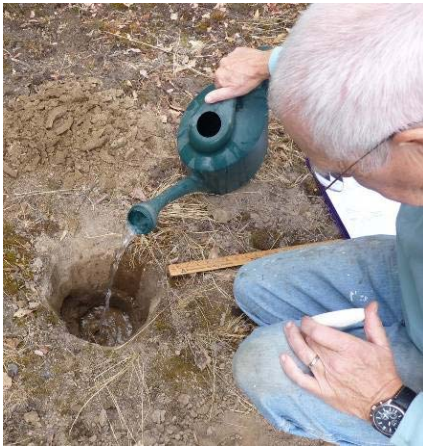
Figure 1 Anyone can perform an infiltration test with commonplace tools.
