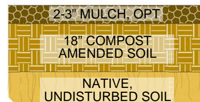
Figure 1 To ensure proper water quality treatment, an 18" layer of healthy soil is needed in all bioretention facilities.
