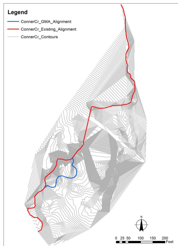
Figure 10 - Alternative 2 alignment. Existing alignment is indicated in red and the Alternative 2 alignment is indicated in blue.
