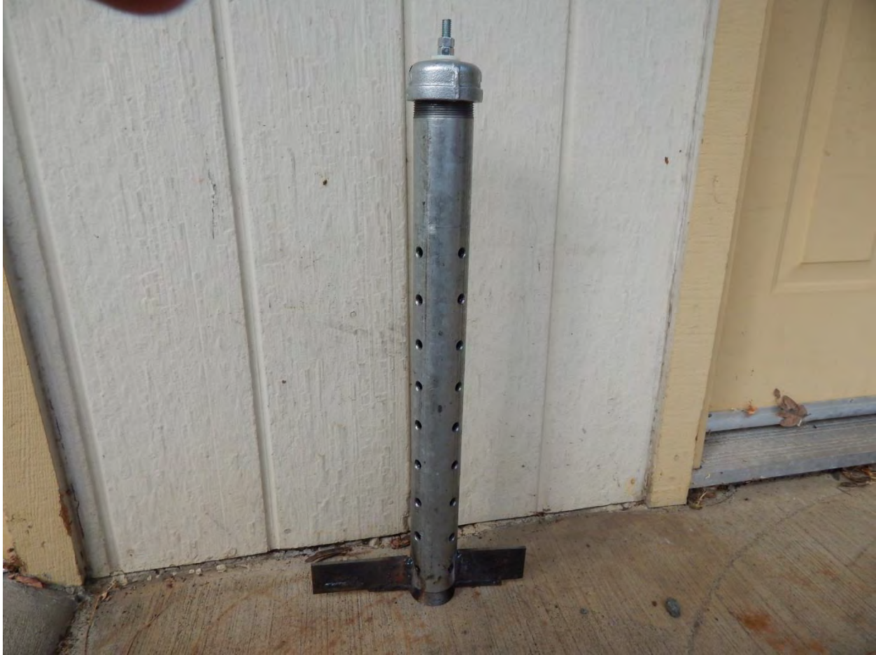
Figure 4. HOBO container for Monitoring Sites #2 and #3.
