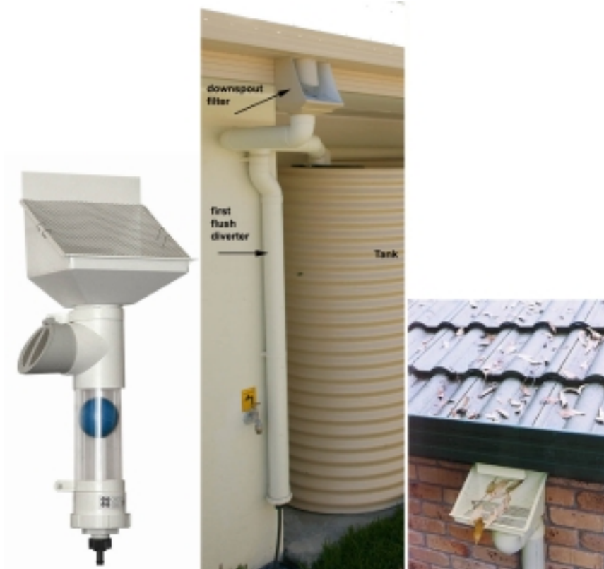
Figure 3. The leaf beater and first flush diverter (left) as a unit and installed into a home catchment system (center). The leaf beater removes leaves and large objects from the water flow before the water enters the first flush diverter (right).
